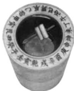
Figure 1 Boussole liquide chinoise
